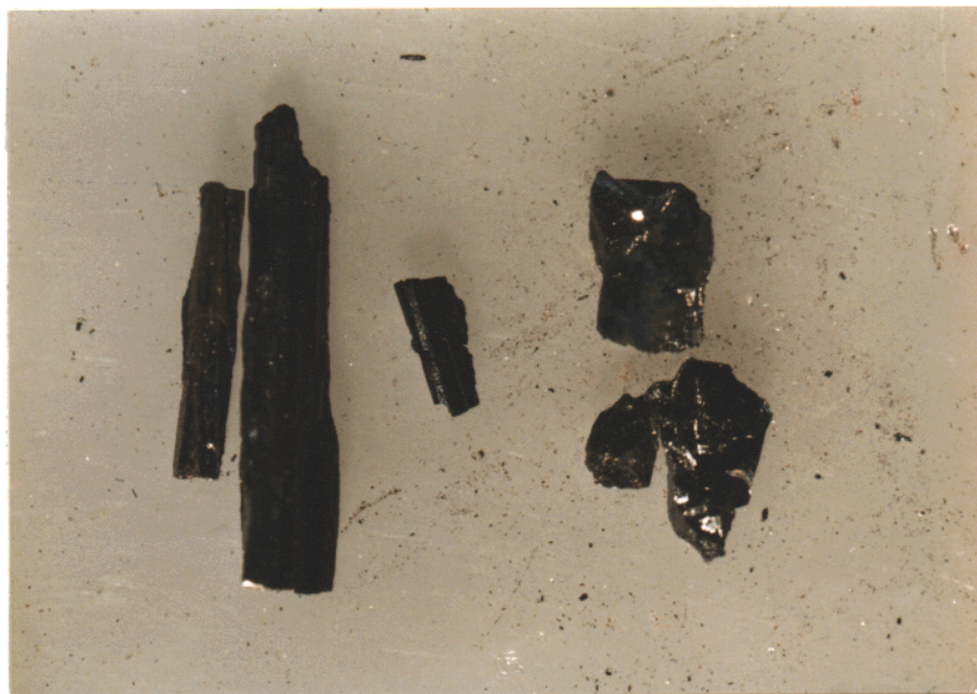
Figure 2. A photograph of TIS crystals; left: the tetragonal TlSe (chain) type; right: the monoclinic TlGaSe 2 (layer) type. Both types of crystal have shiny black colour, but a little different: brownish (chain type) and bluish (layer type).
